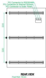
Pixel Pitch: 16 mm Display Color: Amber & White (RGB LEDs) Resolution of Display: 1019 pixels Cabinet Color: Front: Matt Black; Back: Aircraft Grey Max Power Consumption: Approx. 130 W Avg Power Consumption: Approx. 44 W Weight: Approx. 40 KG(Without Battery)
